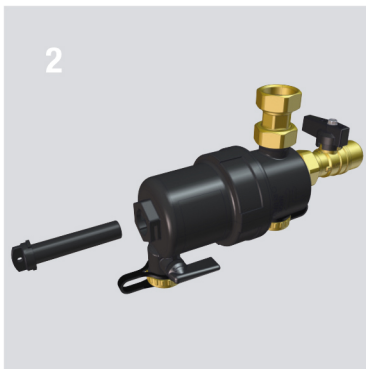
Removing the magnet (turn it 90° clockwise)
